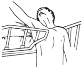
Entrapment between split bed rails
