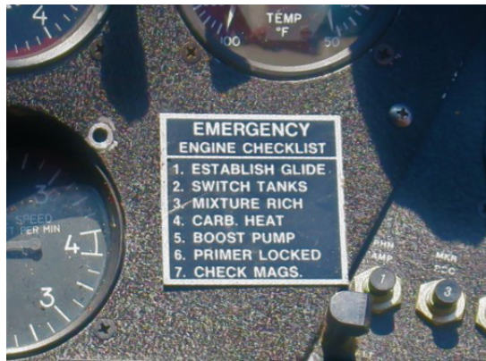
Figure 4: Emergency Engine Checklist plate on board F-GYMF
