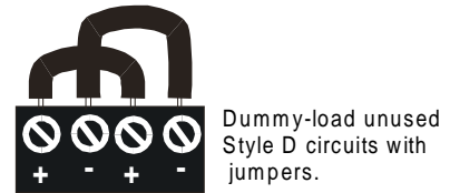
Figure 48: XPM-8 Module (power-limited) with Four Style D Initiating Device Circuits
